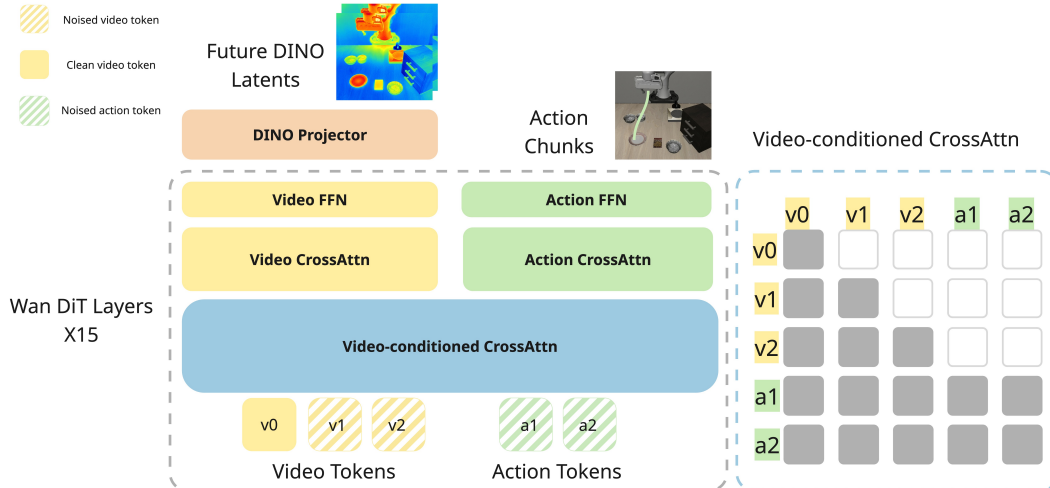
Figure 1: Overview of WanPolicy training pipeline. Some details are hidden for clarity. Left: video-conditioned cross attention and separate cross attention and FFN layers for video and action branch. Video branch is supervised by representation alignment loss with future DINO representation. Action branch is supervised by standard flow matching loss. We read out the features from the intermediate layer of DiTs and discard the later parts. Right: attention mask for video-conditioned cross attention. Video tokens attend to other video tokens but not action tokens. Action tokens attend to both video and action tokens.
