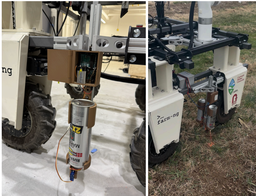
Fig 5. Marking system. Erwin sprays non-toxic paint on the ground to mark infected trees.
